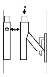
When locking restrictors are fitted, these restrictors may be locked by turning the grub screw (A) anti-clockwise until the end is flush with the face of the restrictor.
